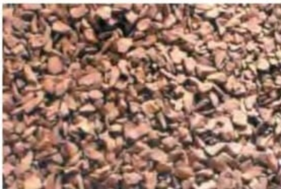
Poorly shaped crushed aggregate. It will make poor concrete.
