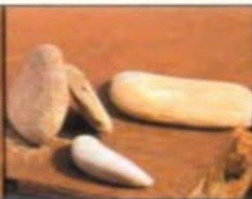
Flaky concrete aggregate.
