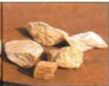
Crushed concrete aggregate.
