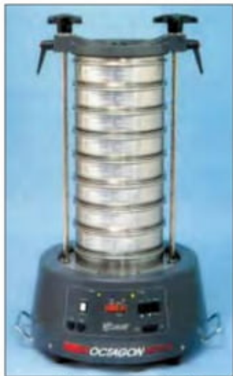
Set of Sieves assembled for conducting Sieve analysis.
