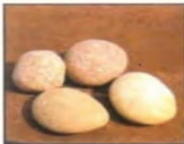
Round (spherical) concrete aggregate.
