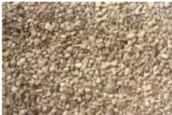
Good aggregate resulted from Barmac crusher.
